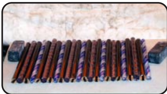
5- When the canes are hot enough to tack fuse they are ready for the roll up.
