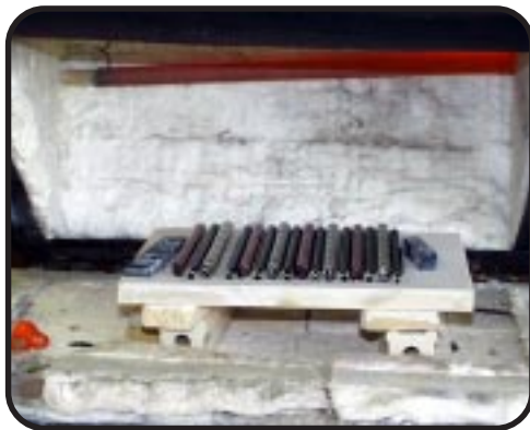
3- A cane lay up is placed in the pick up kiln and heated until they stick together.
